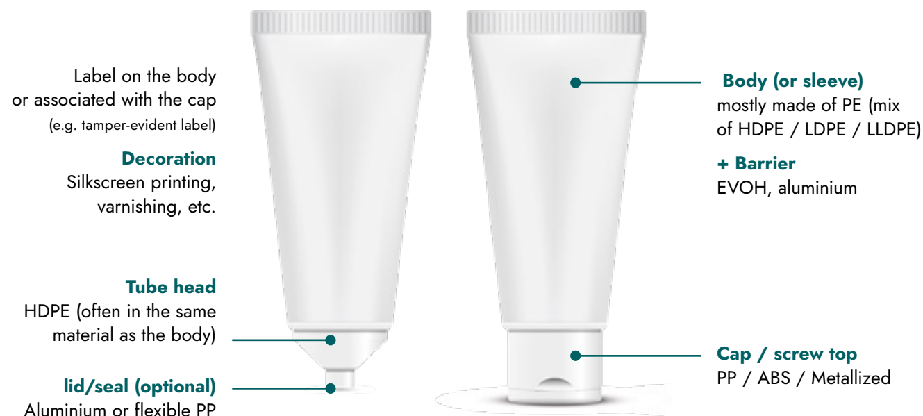
Figure 8: Description of a standard tube made mainly of PE
