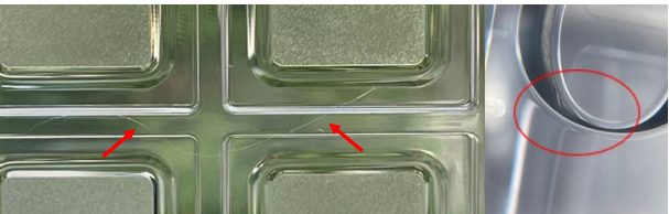
Re-adhesion lines illustration
